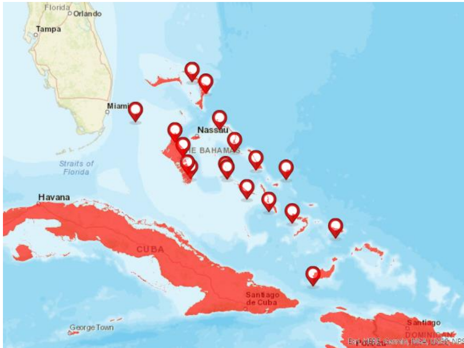
Figure 6. Probabilistic hazard map for Wind Speed (3-sec sustained mean wind speed at 10 meters above water/ground surface – in km/h) for a return period of 500-years. High hazard-classification (in red) consider wind speed values greater than 209 km/h.
