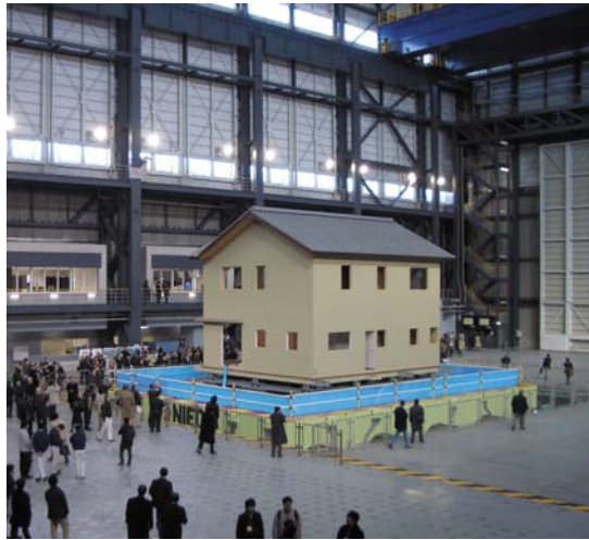
E-Defense Shake Table near Kobe, Japan, ready to test a full-scale house.
