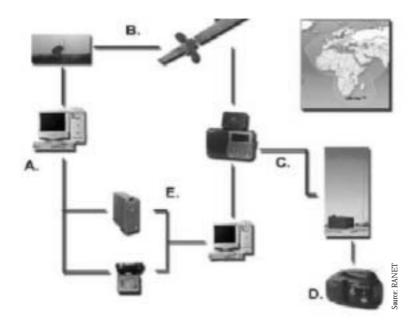
RANET information cycle: Global, regional, national and local information is gathered from various technologies through different methods and then blended in a single broadcasting via Radio existing networks thereby reinforcing local, existing capabilities rather than developing new, resource intensive and unsustainable networks.
