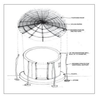
Figure 1. A diagram of the dhani
