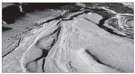
Figure 2. Aerial image of vertical wells in Turpan area of China. Source: www.sunnychina.com
