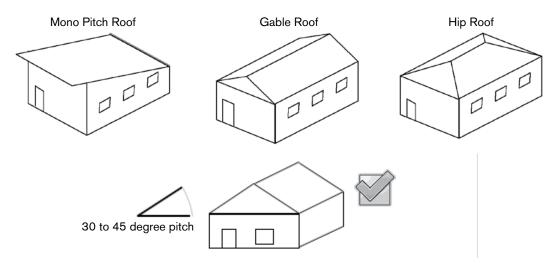
Where roofs of a greater or lesser slope are desired, additional fastening systems should be designed to resist uplift loads.
