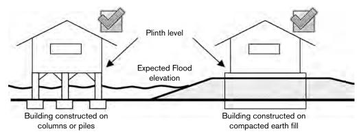
Any technique used to raise the building, must also be designed to resist the forces of standing and moving water and floating debris. Existing buildings can also be raised, although this solution can be costly and difficult. Raising masonry and concrete structures is particularly difficult and can easily damage the building.
