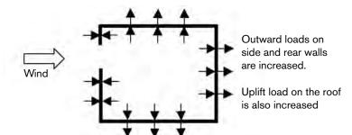
If more air is allowed to pass through the rear and side walls, the building is depressurized and air from within is sucked out of the building. This suction pressure pulls the side
