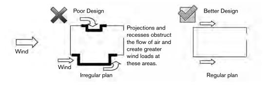
W15. Design and build to resist lateral loads from all directions.
