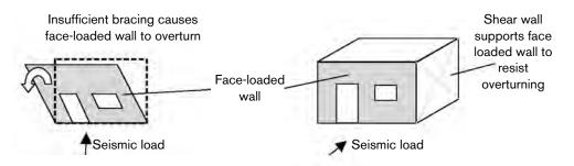
As shear walls help to brace face-loaded walls and stop them from overturning, the corners where they meet should be reinforced.
