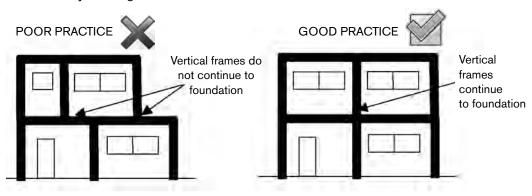
Vertical framing that does not continue to the foundation is a critical weak spot.
