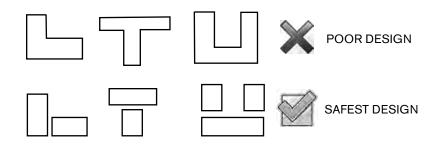
E10. Design building to be vertically regular with respect to lateral stiffness and weight distribution.
