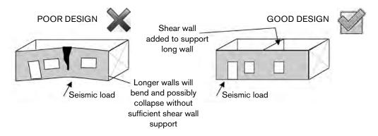
Horizontal structural components which tie all four walls together such as a floor, roof, or upper storey are called diaphragms. Diaphragms further support a face-loaded wall and transfer the load down to the shear walls, or in the case of a floor, directly to the foundation or ground.
