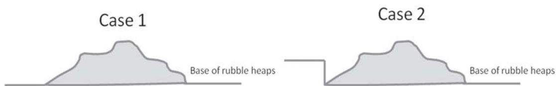
**Fig. 9.** Example of building's base height retrieving. The elevation is estimated from the lower (visible) point adjacent the rubble heap. For instance, in case 2 the lower elevation (right side) is selected.
