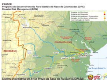
The early warning system is simple but effective. Rain measurements in strategic places of the river catchment are reported to a center located in Buzi. Warnings are issued in case of strong areal precipitation.
