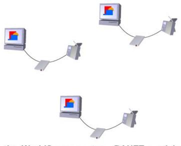
With the WorldSpace system, RANET participants are able to upload their own content to the broadcast via FTP, web forms, and other Internet methods. Even with a very slow connection, critical content can be uploaded to the uplink server. Every hour content is merged into a single presentation that can be viewed by anyone anywhere under the continental-scale broadcast who possesses a WorldSpace receiver attached to an existing computer.
