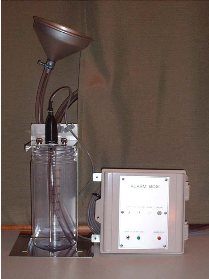
Rainfall equipment with alarm unit
