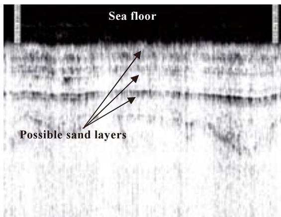
Fig. 3. Sub-bottom acoustic profiling results. Possible sand layers are visible.
