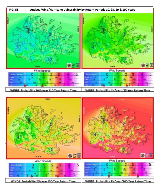
Figure 57 shows a topography map of Antigua identifying the main points of interest – the main town and important harbours. Fig. 58 above indicates the vulnerability of Antigua to winds by the return periods of 10 years, 25 years, 50 years and 100 years (PGDM).
